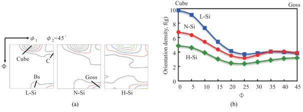
**Fig.7.** (a) The influence of different Si additions on the recrystallization texture evolution. (b) the intensity from the exact Cube component along  $\Phi$  towards the G component of the specimens after fully recrystallization.
