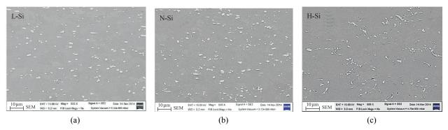
**Fig.8.** SEM micrographs showing the particle distributions of as-PSCed specimens before annealing; (a) L-Si, (b) N-Si, and (c) H-Si.
