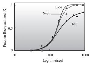
**Fig.4.** Effect of Si additions on the isothermal recrystallization kinetics of Al-Mn-Mg aluminum alloy.
