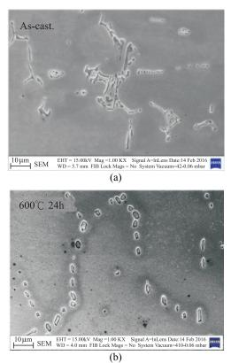
**Fig.1.** (a) Microstructure observations of the primary constituent particle of the Al-Mn-Mg aluminum alloy before, and (b) after homogenization.
