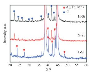
**Fig.2.** XRD patterns of the Al-Mn-Mg aluminum alloy after homogenization at 600 °C for 24h.
