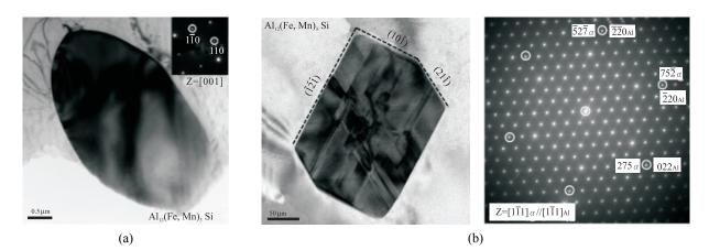
**Fig.6.** (a) TEM analysis of the  $\alpha_c$  dispersoid particles shows high coherency with matrix along [111]<sub>Al</sub> zone axis. (b) The spheroidized  $\alpha_c$  constituent particles.
