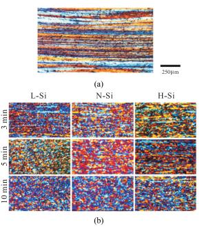
**Fig.3.** (a) Polarization optical micrograph of as PSCed specimen showing the typically elongated grain structure, and (b) the evolution of the microstructure with increasing annealing time.
