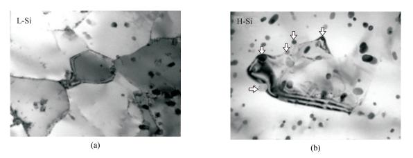
**Fig.5.** TEM micrographs of Al-Mn-Mg aluminum alloy showing the particle distribution varied with different Si additions, (a) L-Si, and (b) H-Si.
